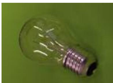
In the incandescent lamp, light is produced by passing an electric current through a tungsten filament contained in an evacuated glass bulb partially filled with an inert gas. The current heats the filament to incandescence. The pressure of the inert gas slows down the evaporation of the filament. Only 3-6 per cent of the input energy results in
